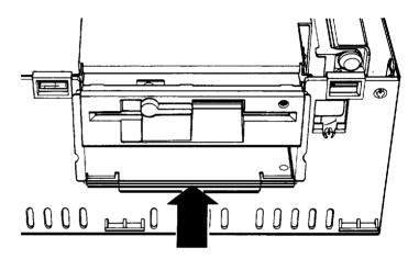
7. Locate the hard disk drive and diskette drive ribbon cables. (The hard disk drive cable is slightly wider than the diskette drive cable.) Check the back of the drives to make sure you know which cable is which.
